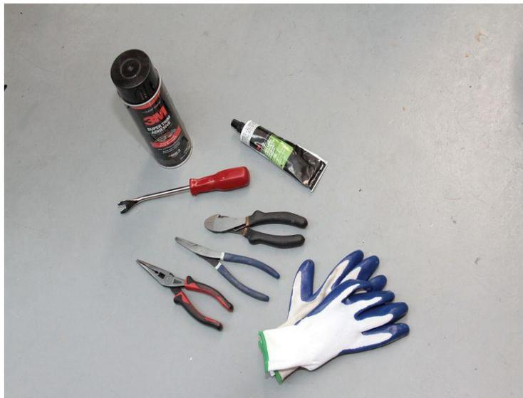
*These are the more basic tools you're going to need to restore seats. You also need to equip yourself with sharp scissors, a razor knife, a tape measure, and silicone spray to ease installation. Don't forget steel hog rings—you're going to need them to secure the upholstery.*
